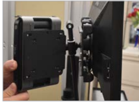
CPU with VQC plate shown being detached from back of monitor.
