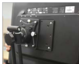
Monitor shown sliding from VQC plate base.
