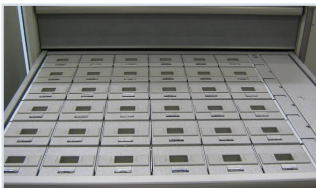
Compartment control lids with pick-to-light guidance
